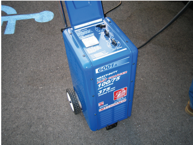
FIGURE 13 A typical industrial battery charger. Be sure that the ignition switch in the vehicle is in the off position before connecting any battery charger. Connect the cables of the charger to the battery before plugging the charger into the outlet. This helps prevent a voltage spike and spark that could occur if the charger happened to be accidentally left on. Always follow the battery charger manufacturer's instructions.
