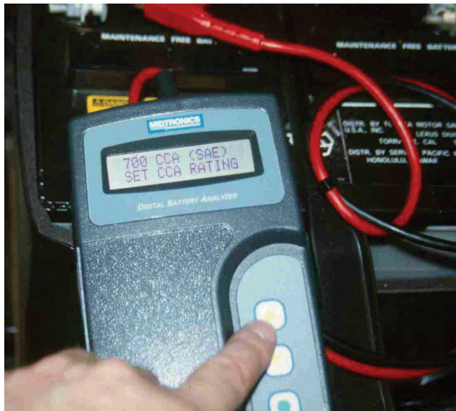
FIGURE 12 A conductance tester is very easy to use and has proved to accurately determine battery condition if the connections are properly made. Follow the instructions on the display exactly for best results.
