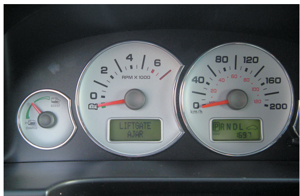
FIGURE 6 The Ford Escape Hybrid instrument panel showing the vehicle in park and the tachometer on “EV” instead of 0 RPM. This means that the gasoline engine could start at any time depending on the state-of-charge of the high-voltage batteries and other factors.
