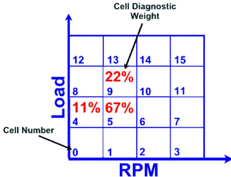
Block cell is the adaptive strategy of the PCM. It's the PCM's ability to learn and to correct for fuel imbalances.
