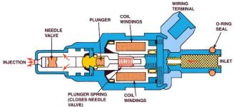
Fuel injectors are a Solenoid used to deliver fuel and are pulsed on to control the air fuel mixture. Injectors are usually energized for 3 to 10 milliseconds. An injector on time of more than 5 ms usually indicates a rich command.
