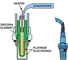
This sensor is used to detect the amount of oxygen left in the exhaust stream after the combustion process. If the mixture is too lean, there will be excess oxygen in the exhaust stream. This will generate a voltage below 0.5 volts. If the mixture is too rich there will be a lack of oxygen in the exhaust stream. This will generate a voltage above 00.5 volts.
