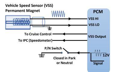
Vehicle speed sensors convert vehicle speed into a digital or analog signal that is sent to the PCM. This information can be used by the PCM for transmission shifting, cruise control, and over-speed control. Vehicle speed sensors can be a Permanent Magnet Generator, or a Hall Effect switch.
