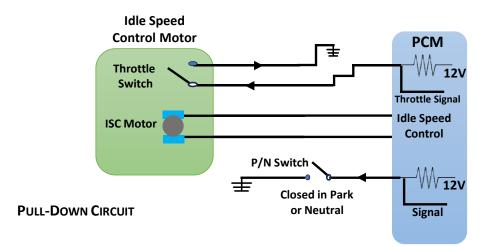
The figure shows two "pull down circuits." These circuits differ from the "pull up circuits" in that the PCM supplies the power, and the switch completes the circuit to ground.
