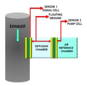
A planar-type wide-band oxygen sensor is made like a conventional planar O2S and is labeled *Nernst cell*. Above the Nernst cell is another zirconia layer with two electrodes, which is called the *Pump cell*. The two cells share a common ground, which is called the reference. There are two internal chambers:
