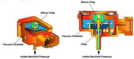
A MAP sensor compares the absolute pressure in the intake manifold to a perfect vacuum. The deflection of the silicon chip is converted to an absolute pressure reading by the electronics in the sensor.
