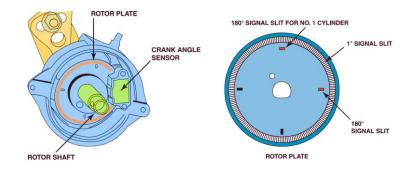
Crank/RPM sensors convert engine RPM into a voltage signal which the PCM uses for RPM, ignition timing, injector timing and over rev control. RPM sensors are also used to trigger the module when controlling the primary ignition.
