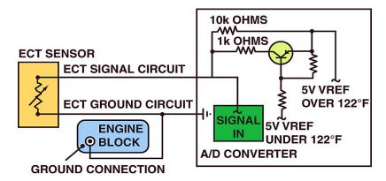
The figure above shows a stepped engine coolant temperature sensor circuit. The purpose of this extra circuit is to give the PCM a more accurate reading of the engine coolant temperature compared to the same sensor with only one circuit.
