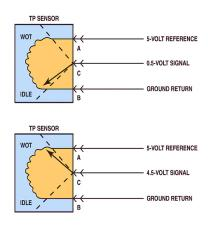
As the wiper moves across the resistor, the signal voltage changes to reflect the throttle angle. The PCM uses this information along with the RPM signal to help determine the proper air/fuel ratio and ignition timing.
