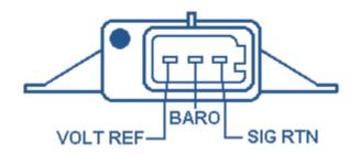
A MAP sensor and a BARO sensor are usually the same sensor, but the MAP sensor is connected to the manifold and a BARO sensor is open to the atmosphere. The MAP sensor can read barometric pressure just as the ignition switch is turned On and before the engine starts. Therefore, altitude and weather changes are available to the PCM.
