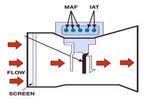
Mass Airflow (MAF) sensors convert intake airflow information into an electrical signal. This information is used by the PCM for fuel delivery and spark timing. MAF sensors will generate either a digital or an analog signal depending on the type.
