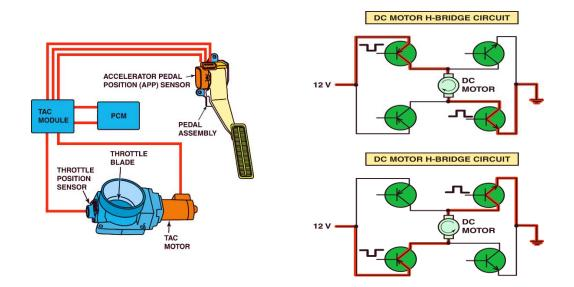
The Electronic Throttle Body motor actuator is a DC electric servomotor. The throttle plate is held in default position by a spring inside the assembly. The Neutral (fail safe) position represents approximately 16-20% throttle opening, which usually results in engine speeds of 1200-1500 RPM. The controller then drives the throttle plate closed or open to achieve idle speeds or speeds higher than idle (acceleration).
